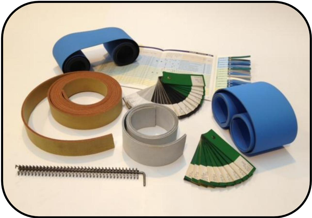
High efficiency synthetic flat belts are currently used in all areas of power transmission, with their light weight construction they lend themselves to being versatile and reliable, with the added benefit of high levels of energy saving.
